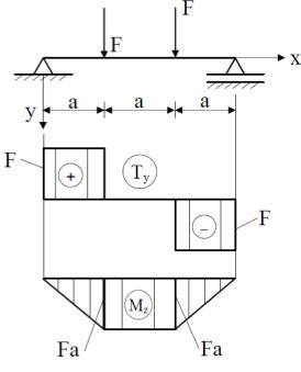
Figure 5. Bending test diagram
